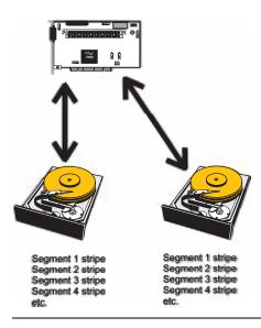
In RAID 1, ADAC Ultra2 S466 duplicates all data from one drive to a second drive. RAID 1 provides complete data redundancy, but at the cost of doubling the required data storage capacity.
